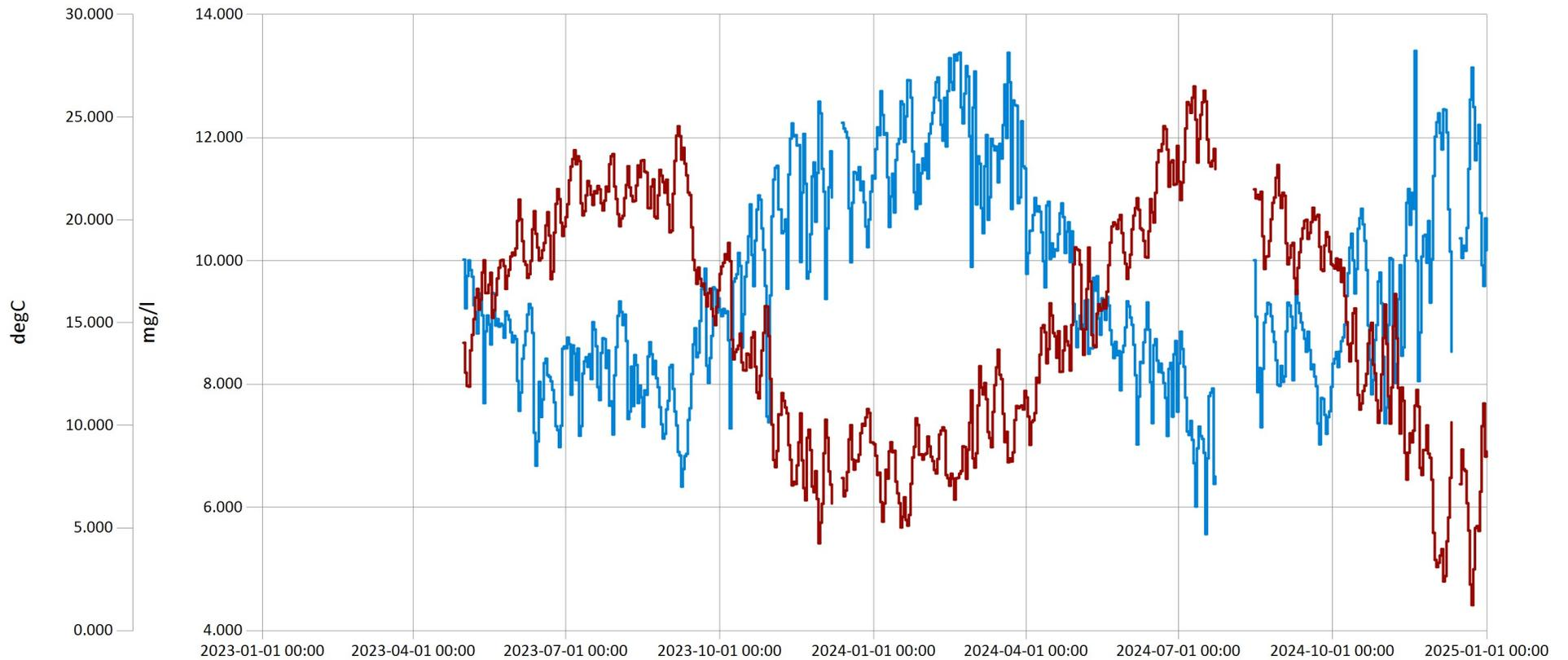
— Dissolved Oxygen (mg/l) — Water Temperature (C)
